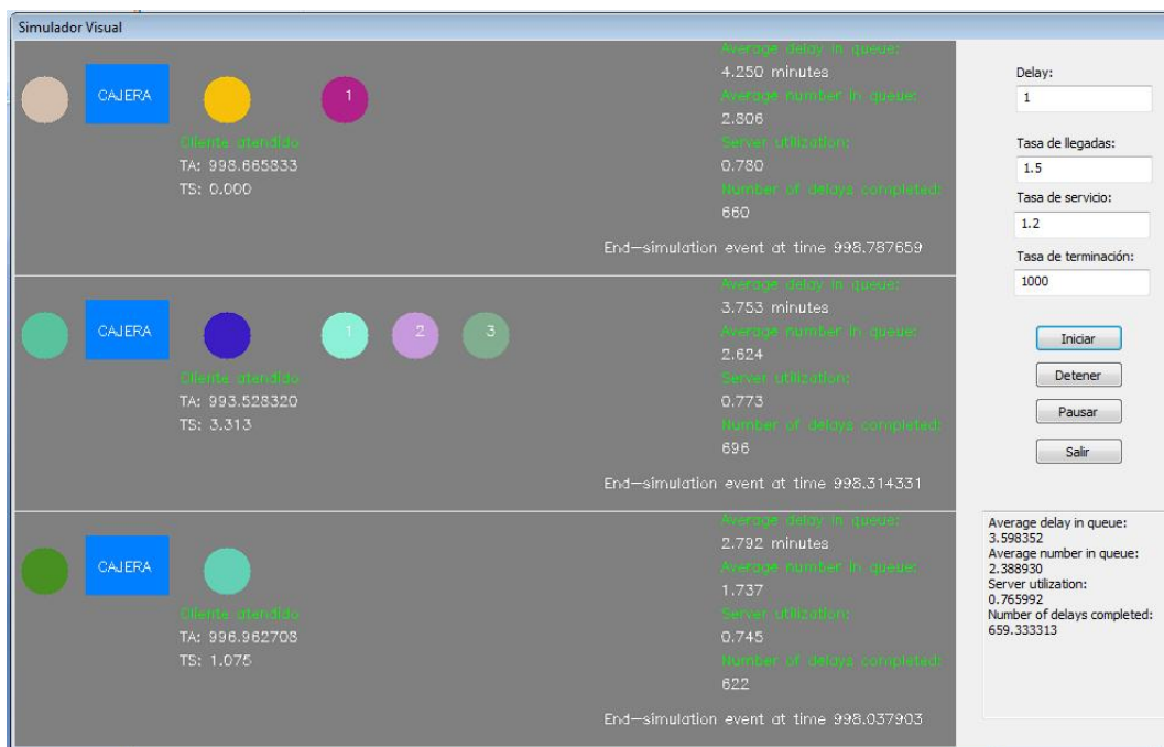
Figure 5. One view of the interface realized for the simulation of the queue supermarket model, here showing three cashiers attending customers (indicated by color balls) and the values of relevant variables. Input data -top right side- are: interval time between customers arrivals and service time. When simulation is finished the output data - left and bottom side-, are: the performance of the system ( \rho ), average waiting time ( W_q ) and expected number of customers in queue ( L_q )
